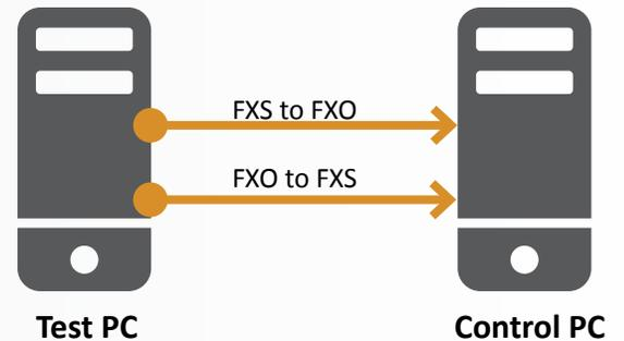
This test utilized a Dell Dimension 3100 running Asterisk with analog interface card modules installed on tested telephony board interfacing with a Digium TDM844B in Whitebox PC running Asterisk.
