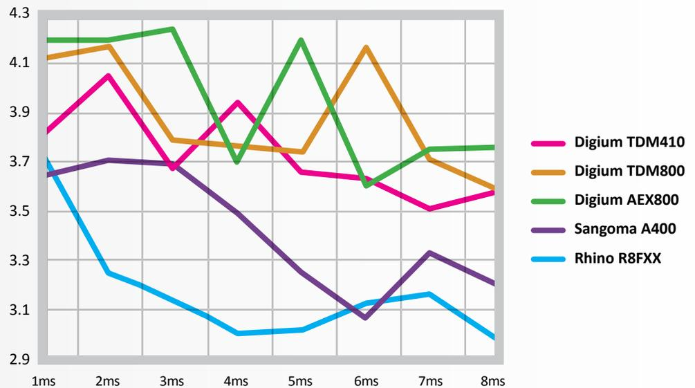
Digium's TDM410, TDM800, and AEX800 cards can maintain their audio quality when interrupts are blocked up to 8ms. Audio quality is acceptable for all interrupt lengths.
