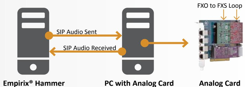
In this test, the Empirix Hammer is used to measure voice quality. It establishes a SIP call to a PC running Asterisk. An analog board with an FXS module looped to an FXO module is installed in the PC. The call is routed, by Asterisk, through the analog modules and then back to Asterisk where it is then passed in SIP to the Hammer.
