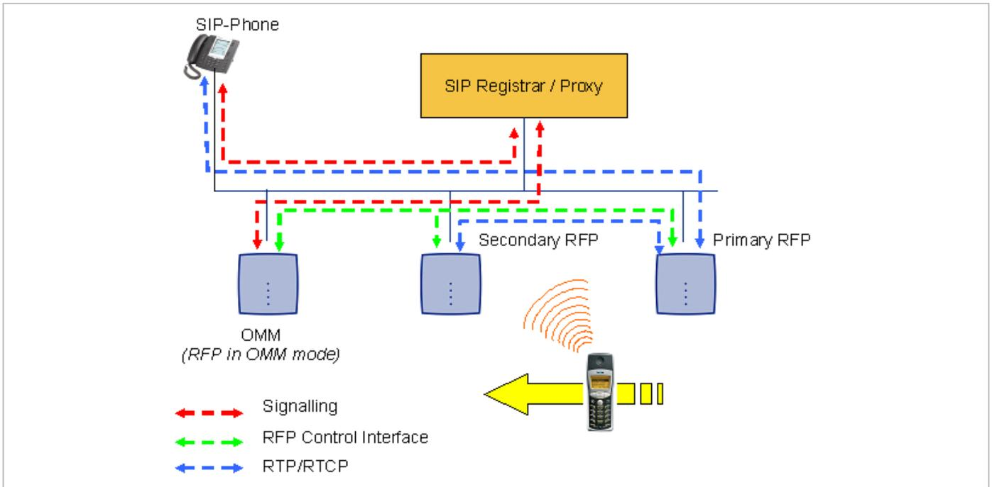
As the DECT phone user moves into the next RFP zone of coverage, the DECT phone detects that the RFP has a better signal strength. Again the media stream from the SIP phone cannot move to the secondary RFP, so the primary RFP uses the LAN to direct the voice to the new secondary RFP.
