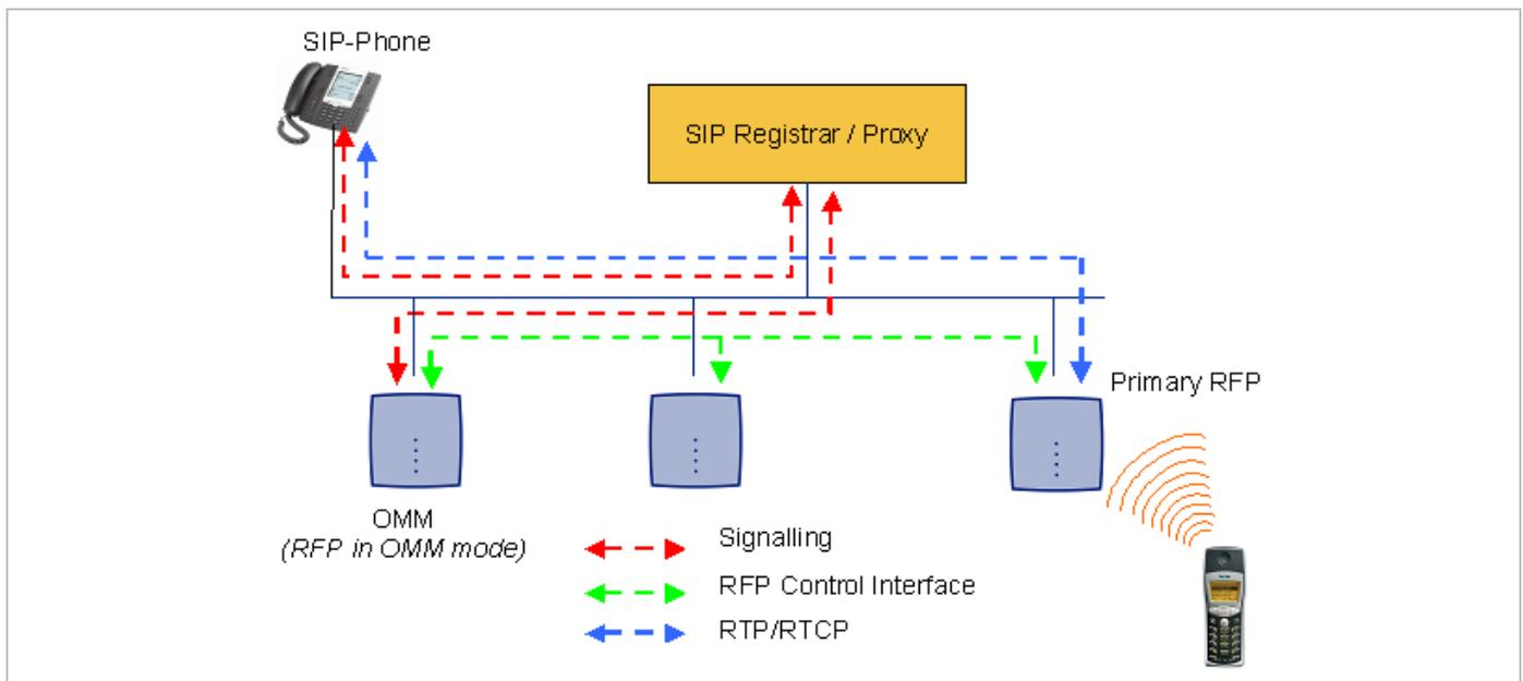
To establish a call between two DECT phones, the same IP streams must be established like in the scenario before, except the IP phone is not involved. The following figure illustrates this scenario.
