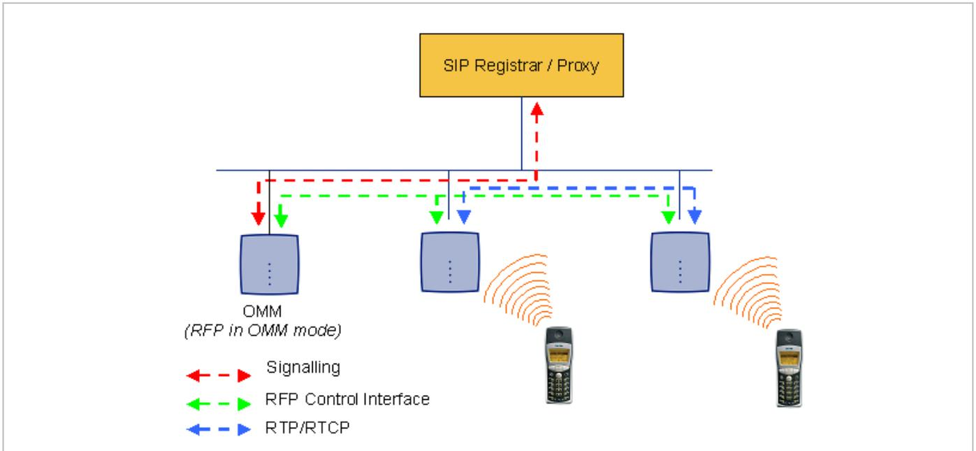
A call from one DECT phone to another that resides on the same RFP will loop back within the RFP if no media gateway is involved. So the call will not pass through to the Local Area Network (LAN). Although the voice packets will not impact LAN traffic, signal packets will.
