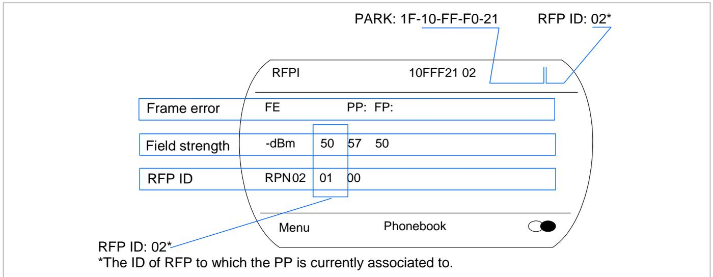
In this example the DECT phone is currently connected to the RFP with the number 02. The RFPs 01 and 00 are also visible. The number "10FFF21 02" on the upper right side refers to the PARK (Example 1F-10-F2-21) of the SIP-DECT system and to the RFP to which the phone is currently connected to.
