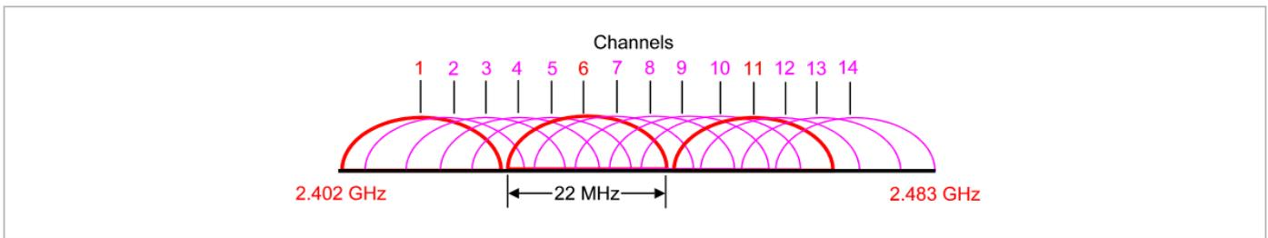
When planning the radio coverage for a two-dimensional area, please bear in mind that the distance between any two base stations operating on the same frequency must be at least twice their range. The range can be adjusted by lowering the output power level.
