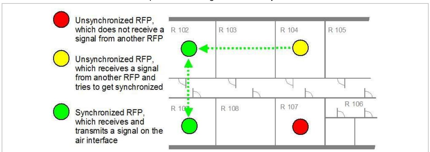
As long as a DECT base station is not in sync, no calls can be established using this DECT base station. If a DECT base station loses the synchronization, the DECT base station does not accept new calls (“busy bit”). There is a delay of maximum 3 minutes until the active calls on this DECT base station are finished. Then it tries to get synchronized again.
