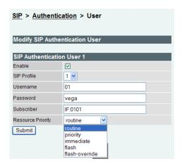
The resource priority is configured through the selection of an entry in a pull down box. The values contained in the pull down box are the values defined in the NameSpace configuration (see section 15.6.1 "Configuring NameSpace for").
