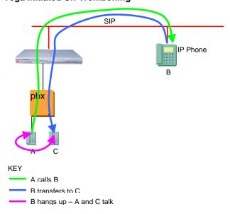
The Vega's default behaviour relies on detecting that two SIP call legs have the same call ID in order to initiate the QSIG side un-tromboning. Other headers can be checked and verified using the following parameters:
