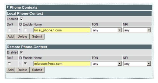
**Local Phone-Contexts** are used to populate the From header for ISDN to SIP calls based on the values of TON (Type of Number) and NPI (Numbering Plan Information) in a received ISDN SETUP message. They are also used to set the values for TON and NPI in the called party number IE in the outgoing ISDN SETUP when a matching phone context is received in a SIP INVITE.
