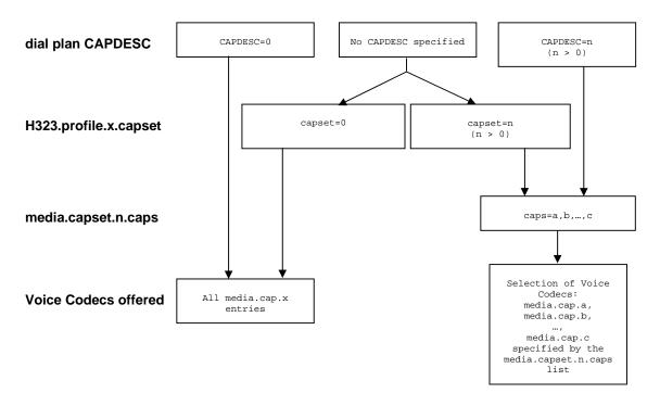
In the dial planner a token CAPDESC: can be used (in a dest statement where the interface is IF:0501) to specify which codec set (media.capset.n.caps list) is to be used to specify the list of codecs to offer (and their priority order).
