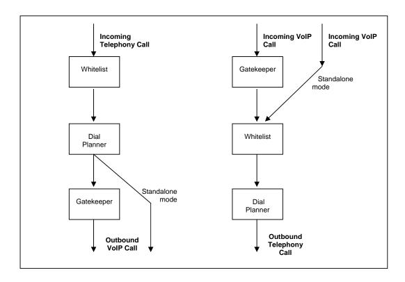
To select the mode of operation configure h323.gatekeeper.enable on the CLI or select the appropriate "Gatekeeper Mode" or "Standalone" button on the H.323 page on the web browser interface.
