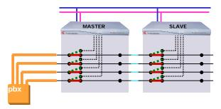
The status of the ISDN fallback relays can determine whether SIP registration takes place on a Vega 400 (models where ISDN fallback relays are fitted).
