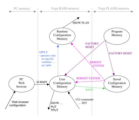
Only parameters in the user configuration memory can be viewed directly in their raw stored form. When information is displayed from the run time memory, for example using commands
